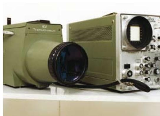
*The first thermal imaging cameras were bulky systems that needed to be filled with liquid nitrogen*
